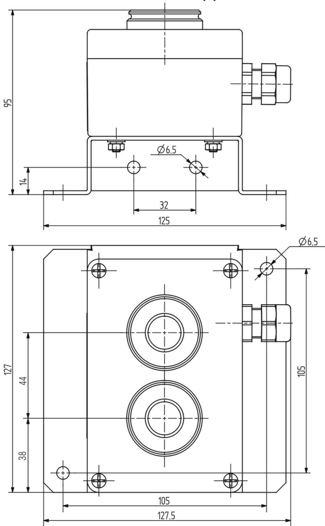
*Dimensions of IR-NE-3 transmitter with pipeline connectors for sampling system applications*
