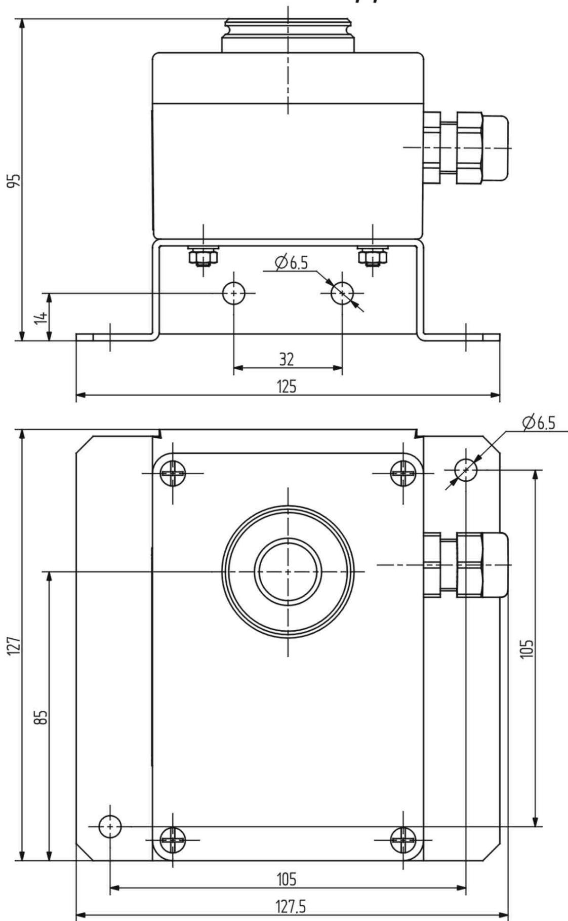
*Dimensions of IR-NE-1 transmitter with pipeline connectors for sampling system applications*
